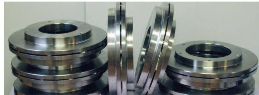
Zvarené obežné kolesá turbokompresorov/Welded turbocompressor runners
