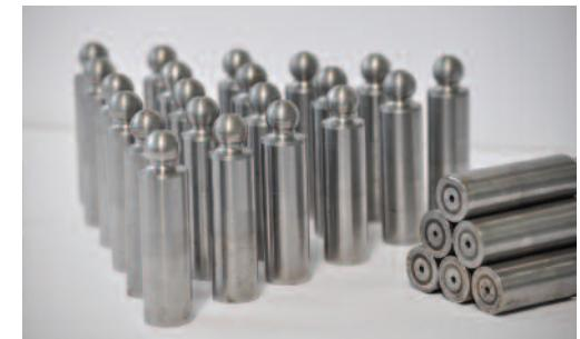
Zváranie piestíkov hydromotorov/Welding of hydromotor pistons
