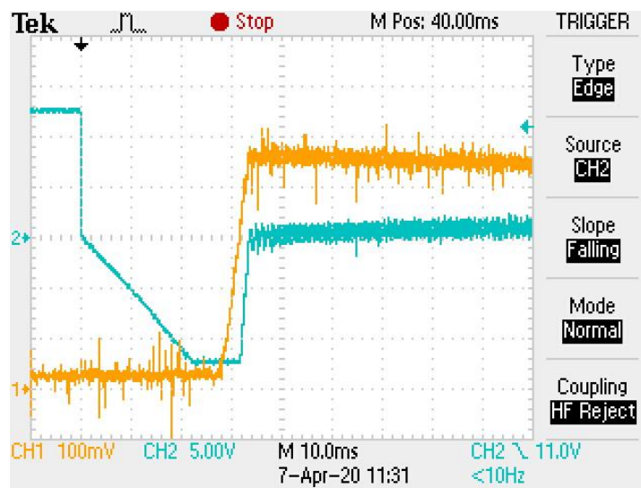
Fig. 4 Start of the welding current I_z = 50\text{mA} , the course of the measured value and the output voltage of the regulator with higher control dynamics
