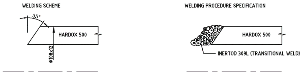
Fig. 4 Schematic of the transitional weld joint
