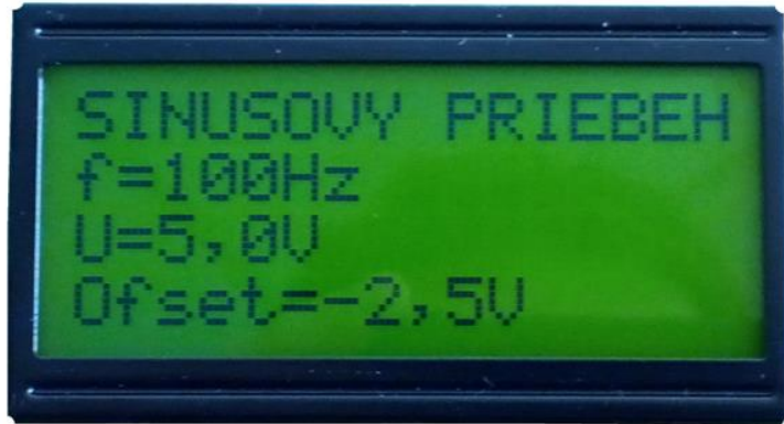
Fig. 3 Display of set parameters a) 2x8 characters b) 16x4 characters
