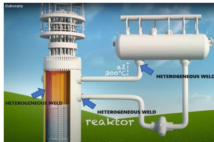
Fig. 1 The primary circuit diagram of a nuclear power plant
